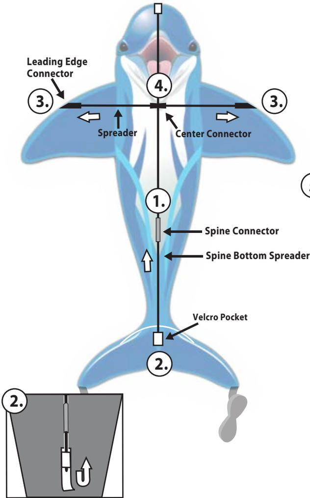
1. Connect Spine Bottom Spreader into Spine Connector.
